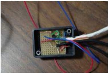
The blue and red wires connect to the GPIO pins on the RPi that control PTT. The black cables go to the Mic and Speaker jacks on the USB sound card. The white cable connect to the Speaker and Mic jacks of the 2m radio. I didn't include any isolation for the audio lines and haven't had any problems, but the box has room, if I decide to add it later on. There is also room to add a transistor and resistors for a COR line to GPIO pin, if desired. I am using VOX instead.
